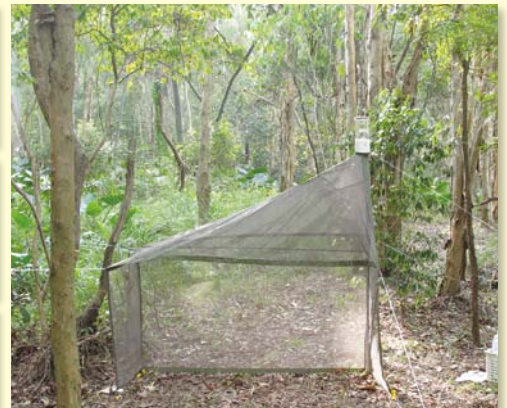
馬來氏採集器的網上可採集到不同的昆蟲 Malaise trap collects insects which had met the mesh of the trap
